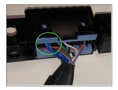
**Incorrect Configuration:** Note, the Larger, blue wire goes into the first pin slot counted from right to left. The wire should be going into the 7th position, where the brown wire is located on this photo
