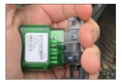
3. Connect the extended blue cable that comes from the monitor extension cable to the power source that provides voltage when the rear hatch is opened.
